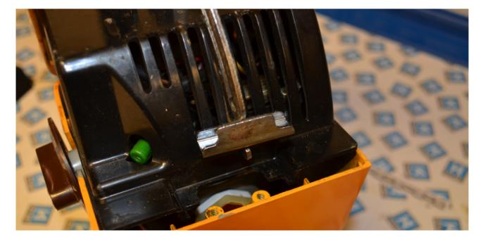
I then suggest taking this metal plate off as well as it will make it easier to remove the vented body cover.
