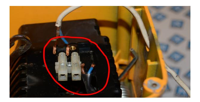
Here I have highlighted where the wires have pulled out. You can also see that the screws haven't been unscrewed fully to get the wires out.
